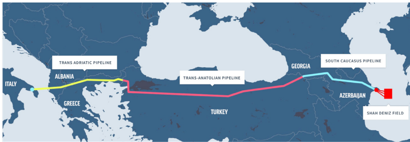
Southern Gas Corridor: SCPX (current 24.04 bcma, with up to 31 bcma extension capacity), TANAP (current 16.2 bcma, with up to 31 bcma extension capacity), TAP (current 10.5 bcma, with up to 20 bcma extension capacity by 2027),
